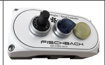
Fischbach setpoint adjuster HF10F IP66 with blue LED toggle switch 0-I and additional yellow LED indicator light contains a 10 kOhm potentiometer for controlling devices with 10V output or 0-10 V control input, as well as an additional switching contact for valves etc. Robust, impact-resistant surface-mounted housing, protection class IP66.
