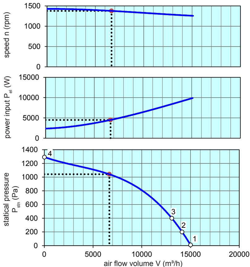
max. permissible ambient temperature from point 1-2: don't use in this area
