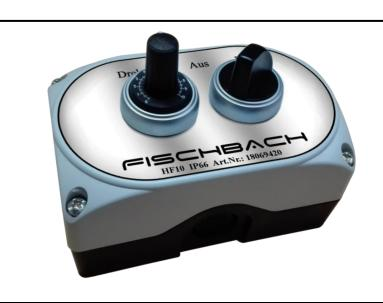
The Fischbach control unit HF 10 IP 66 with toggle selector switch 0-I includes a 10kOhm-setpoint adjuster for controlling units with 10V-output and 0-10V control input, as well as an additional switching contact. Solid, impact-resistant surface-mounted casing, protection class IP66 for use in industrial and kitchen areas.
