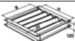
Damper type „A“: for total cross section of unit 662 mm width (B) x 662 mm height (H)
