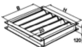
Damper type „A“: for total cross section unit 900 mm width (B) x 310 mm height (H)
